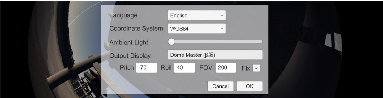
3. Set Pitch, Roll, FOV, and Fix according to the projector and dome shape to be projected.
